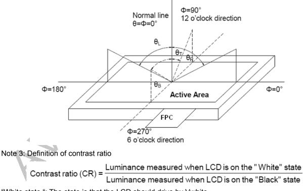
"White state ": The state is that the LCD should drive by Vwhite.
