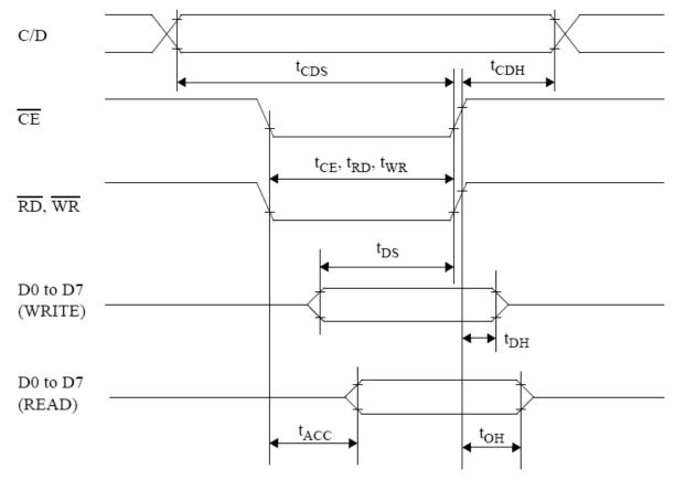
Test Conditions(Unless Otherwise Noted, VDD=5.0± 10%, Vss=0V, Ta=-20 to 75°C)
